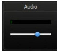
The Audio Input meter displays the audio level for the recording. The best audio quality occurs when the Audio Input meter is in the green to light orange range. Audio clipping may occur in the mid-orange to red range. Drag the slider to adjust the audio. See **Troubleshoot the Volume Level**.
